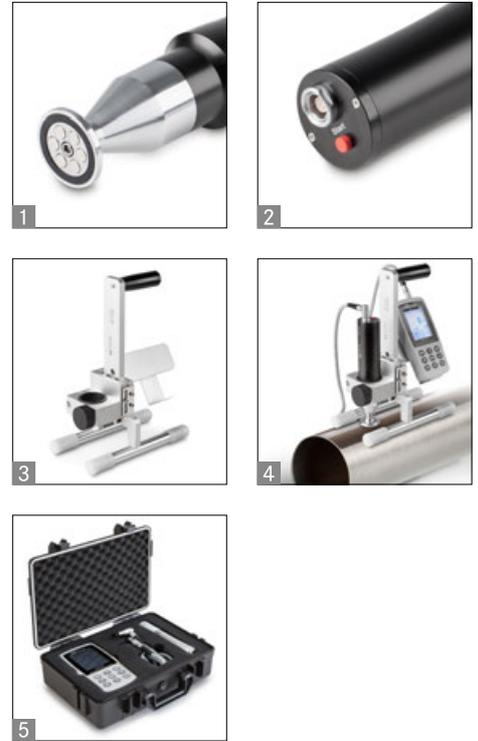
Premium UCI hardness testing device for Rockwell, Brinell and Vickers with a motorised sensor for automated measurement processes
